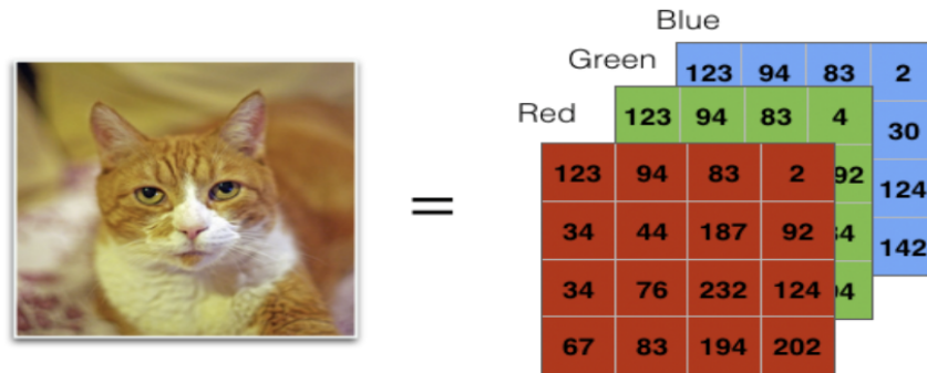
Figure 3: Natural images are represented in a computer as tensors of order 3 with pixel intensity values across color channels. Scheme borrowed from Andrew Ng CNNs course materials.
